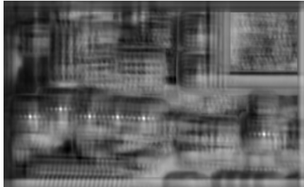
Figure 7.2: Example template correlation image. Each pixel takes a value between -1.0 (black) and 1.0 (white).
